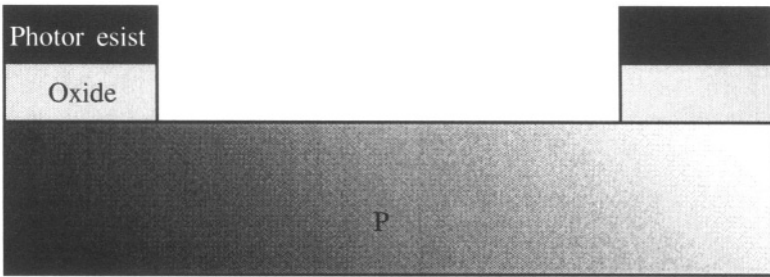
Figure 11.27c: Photolithography and oxide etch to define the buried collector.
